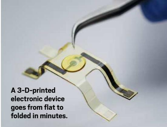
A 3-D-printed electronic device goes from flat to folded in minutes.
